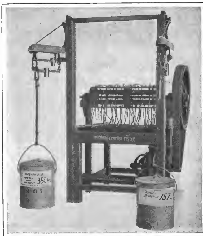
Machine for testing tensile strength and surface durability of leather, etc. A strip of Fabrikoid suspends the pail at the left, which contains 350 lbs. of sand. The strip of split leather suspending the pail at the right broke at 157 lb. pull. The beaters, attached to the rack revolved by belt from the electric motor, play on parallel horizontal strips of Fabrikoid and split leather. The results of this test are illustrated on page 270
